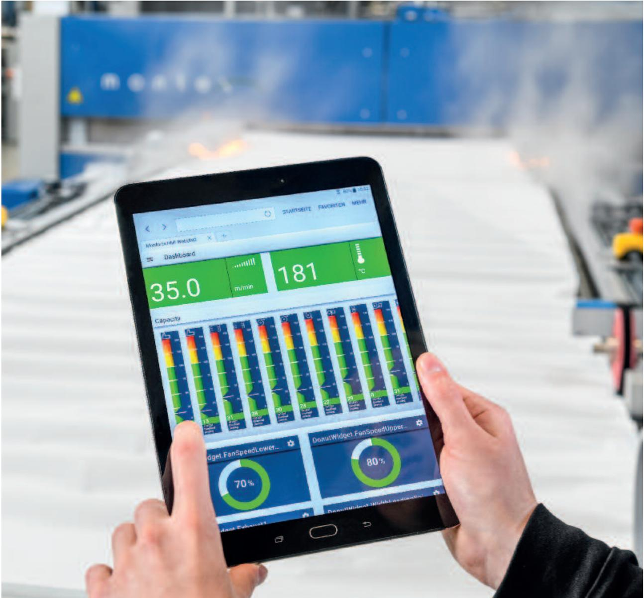
The application "WebUI" by Monforts offers live streaming of machine-data, actual and historical alarms as well as network-camera feeds of Monforts machines. As a software based on HTML5 it can be used on any kind of mobile device (such as cell-phones and tablets) or PCs - as it can be accessed by any browser, no installation of software is necessary. When connected to the internet, the software (running on the machine PCs) can even offer a worldwide overview of the actual status of machines.
